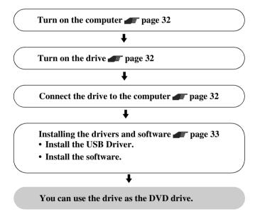
When you install the supplied driver and software in various driver and software, follow the above procedure.
